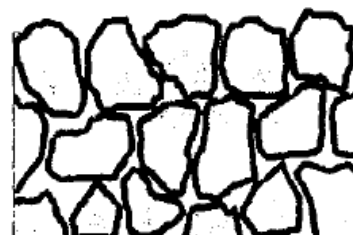
Porous Asphalt (Open Graded Friction Course)
